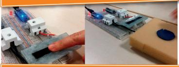
Capacitive and resistive activation properties integrated in any surface type (e.g. plastic, foam, textile, paper, film)
